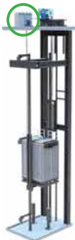
Machine Room Drive on the Rooftop
